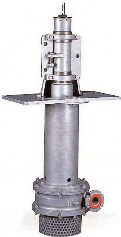
1. Vertical cantilever pumps have no 'wetted' bearings, as bearings are mounted above the mounting plate allowing the ability to run dry, resulting in minimal maintenance.
