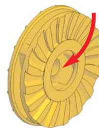
Front vanes. The impeller front shroud has profilled pump-out vanes that reduce recirculation and increase wear life.
