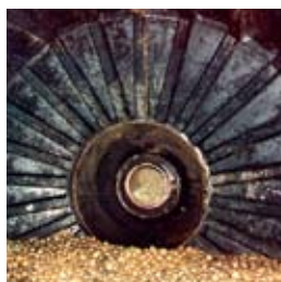
Bottom left: Interior of a Vulco® rubber lined ball mill
