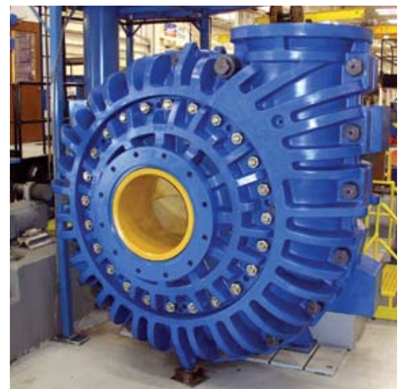
The 600 HTP being prepared for hydraulic testing. The massive casing reinforcing ribs and 102,000 lb bare weight illustrate the robust design and inherent safety.
