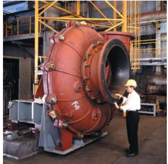
The 1000TY GSL pump incorporates the newest molding technology using a continuous FRP support shell along with internal steel stiffening to support the thick rubber liners. This provides an extra support base to resist vacuum and provide longer life to the liners.
