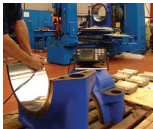
(Top) Weir Minerals Services white metal foundry. (Centre) White metal machining. (Bottom) Ultra-sonic bond testing. (Left) Finished steam turbine bearings.
