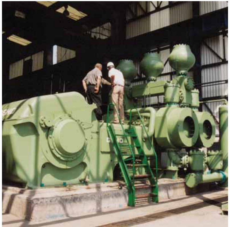
Top left: The Netherlands, propeller pumps for brine circulation
