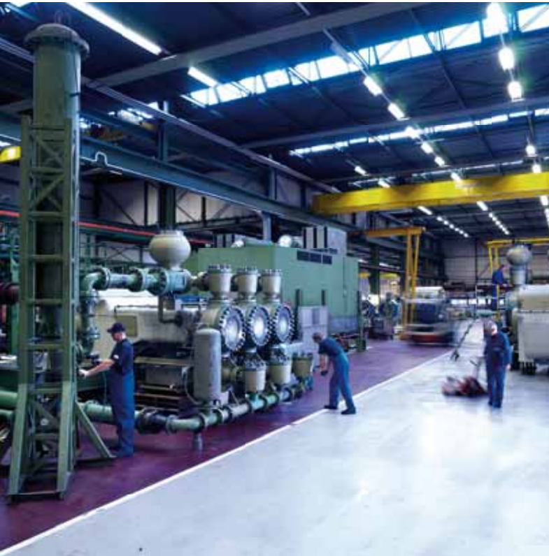
Modern well-equipped test stand for pump tests in real operating conditions
