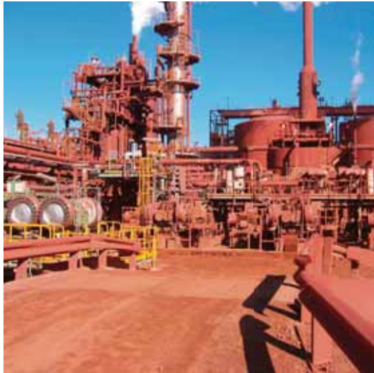
Right: Australia, autoclave feeding of 200°C nickel slurry
