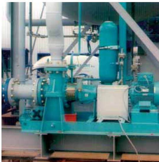
Left: API centrifugal pumps for the oil and petrochemical industry
