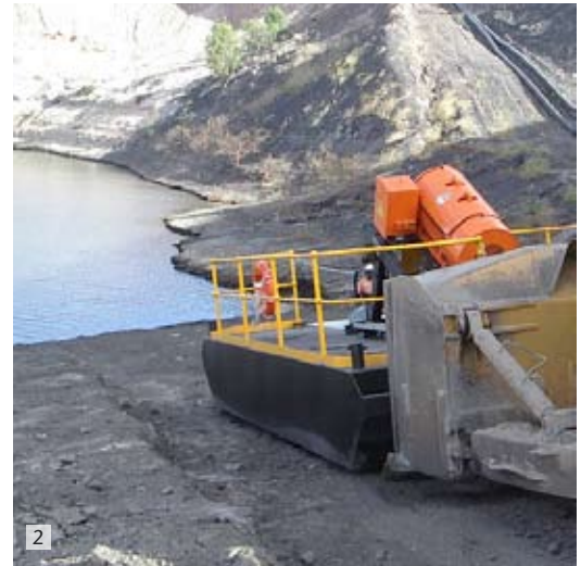
1 : Hazleton vertical cantilever with 800HP motor on 11' pontoon 2. Multiflo pontoon unit skidded around mine site 3 : Single and double pontoon pump unit operating in tandem 4 : Vertical pump on poly float pontoon
