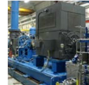
Left and below: Witness testing a 20-30 CTC slurry pump
