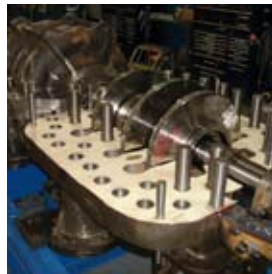
Left: High pressure slurry pump up to eight stages
