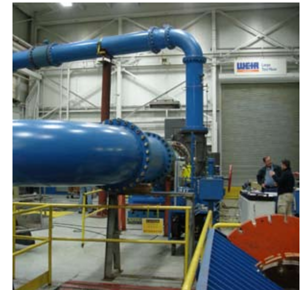
Above: Slurry pump mounted on API base plate
