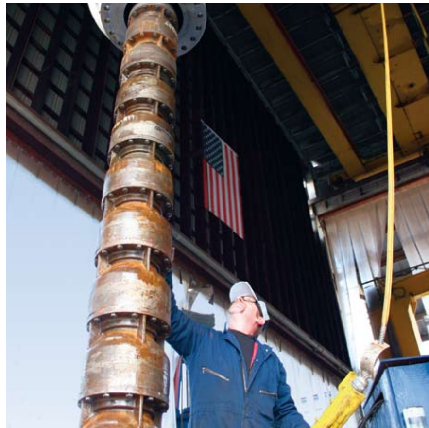
From below left to right: Stainless steel impellers Bowl assemblies Floway pumps state of the art testing facility
