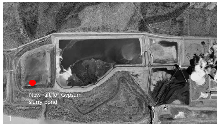
1. Overhead view of the generating station's Gypsum slurry pond. The large pond next to the GSP is the Bottom Ash Pond that is undergoing expansion.
