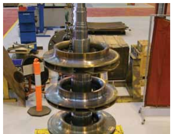
(Top) Workshop refurbishment of screw rotors. (Centre) Radial compressor site inspection. (Bottom) Compressor shaft assembly in workshop. (Left) Finite element analysis of compressor impeller.
